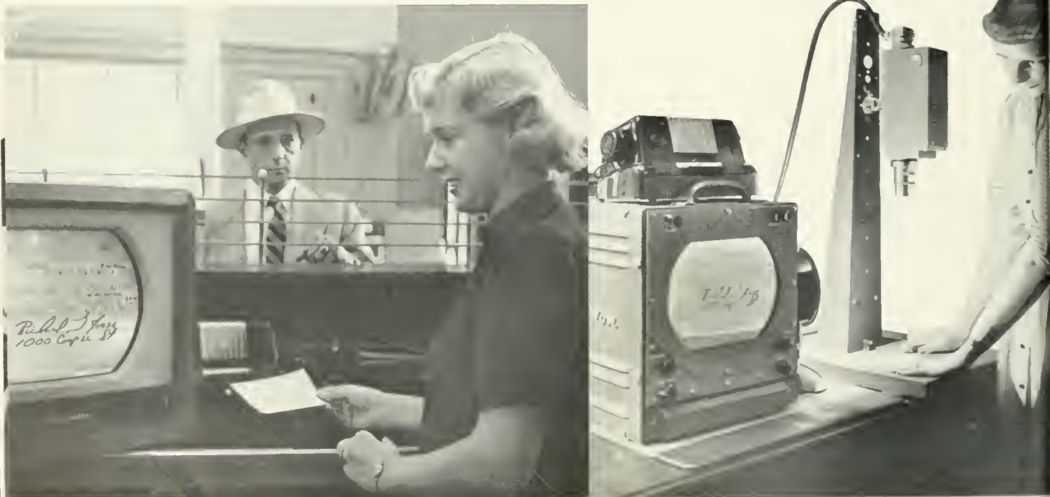
Bank employees use an RCA Industrial Television System to compare signatures on checks and other documents.
