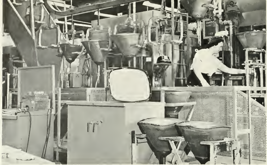
Rapid public acceptance of metal-shell kinescope picture tubes keeps production lines busy at RCA plant, Marian, Ind.
